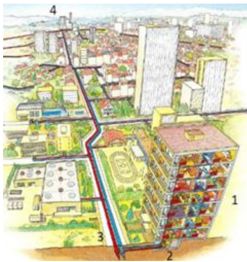
Figure 1 A District Heating Distribution Network (DHN) (Werner S. , 2013)
